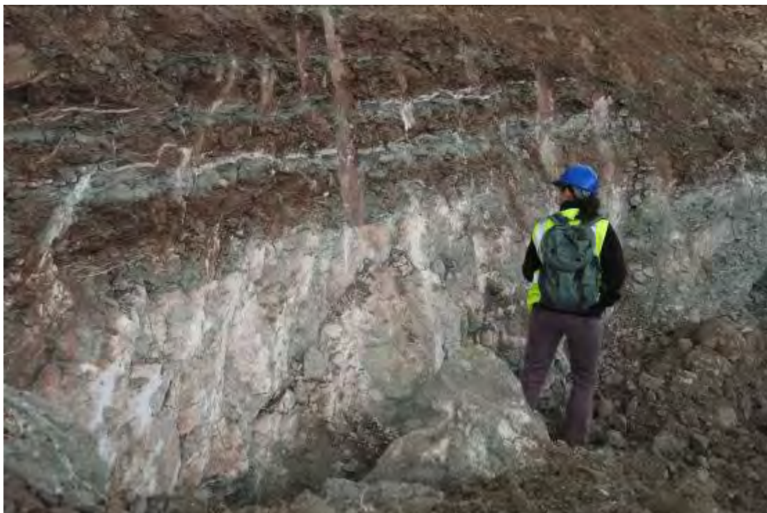
Photo 3: A closer view of Cocks Seam: note thin strings of secondary fibrous gypsum, or satin spa, above the principal seam.
