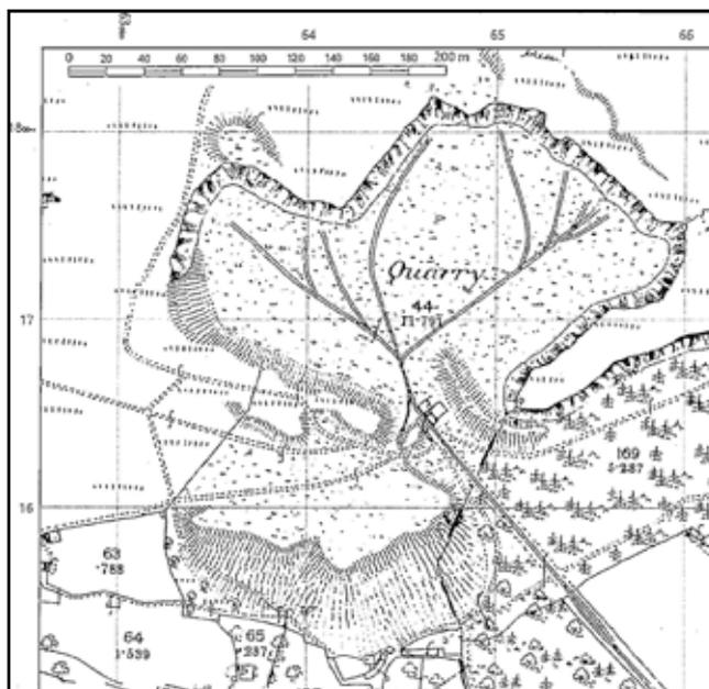
**Figure 12.** Ordnance Survey map of the Welsh Quarry (Chirk Castle Estate) at Llanymynech Hill, published in 1874 at 1:2500 scale. The top of the cable-worked incline is at the drum house (square outline). Tramways (two-foot gauge) within the quarry lead to the incline top. The large flat-topped tip of waste material below the main working floor, south of the quarry entrance, is visible in the landscape today.
