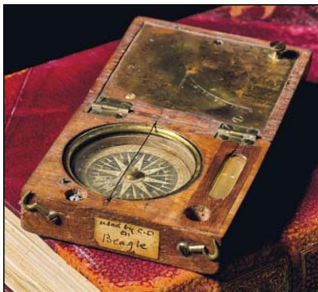
**Figure 5.** Darwin’s compass-clinometer made to a modified design by Henslow in mid-summer 1831. It is currently on display in Down House, Kent. This was subsequently taken by Darwin on H.M.S. *Beagle* (photo: English Heritage).
