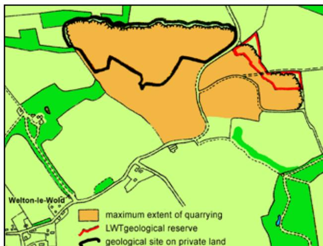
**Figure 10.** Locations of the two quarries at Welton-le-Wold. The road between the quarries follows a small Devensian meltwater channel, and roughly lies at the limit of Devensian ice advance from the east. LWT = Lincolnshire Wildlife Trust.
