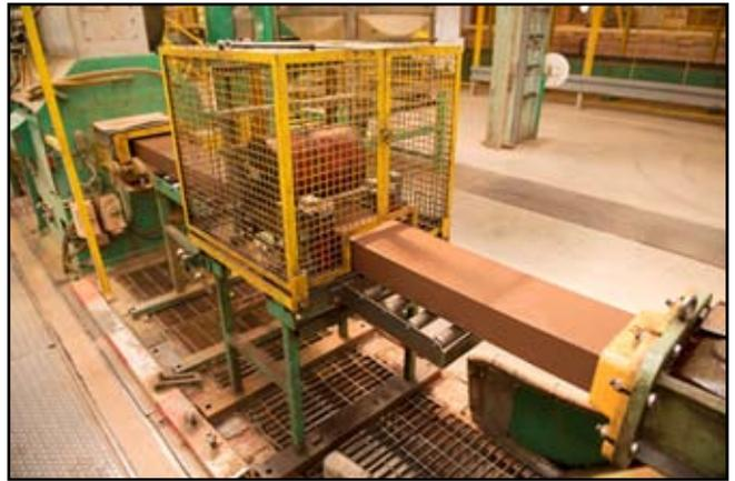
*Moulded clay extruded as a single strip prior to cutting into brick-sized blocks ready for to go into the kiln.*
