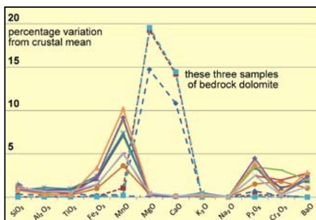
**Figure 5.** Chemical analyses of ten samples of the wad and three of the dolomite bedrock, compared with mean values for upper continental crust.
