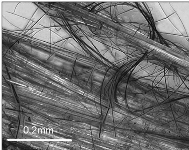
**Figure 2.** Curled fibres and fibrils of chrysotile, seen under an optical microscope (Photo: Barbara Cressey)
