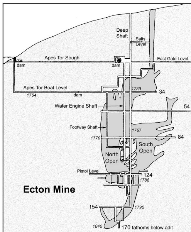
**Figure 1.** Diagrammatic section of the Ecton pipe, redrawn after a mid-19th century prospectus; numbers in the larger font indicate depths in fathoms below adit level at the Apes Tor Sough, and numbers in the smaller italic font indicate dates of the advancing workings.
