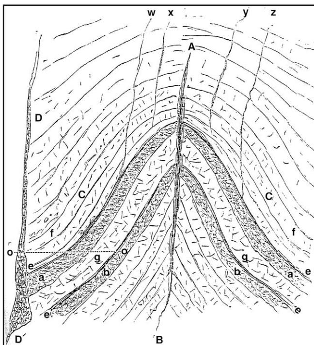
**Figure 2.** Joseph Watson's 1860 diagram of a saddle (reproduced from Porter, 2004, page 21). A is the crown or huckle of a saddle; A-B is the saddle joint; C and C are the wings; D-D is a trough joint, usually more productive of ore than a saddle joint; w, x, y and z mark fissures, which ran up to a pipe vein; f and f are troughs rich in ore, particularly at a and a; e and e are soft decomposed limestone, taken to be guides to ore; o-o marked a cross-cut to reach the wings and troughs.
