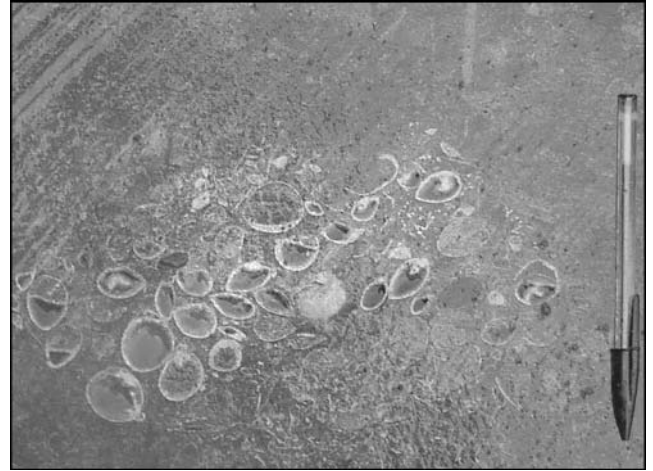
Figure 9. Sawn slab of 'Hornton Stone' (Pliensbachian possibly up to Toarcian Marlstone Rock Formation) at Edgehill Quarry RIGS (SP372468). Note the 'nest' of predominantly fully articulated terebratulid brachiopods. Scale is provided by pen.
