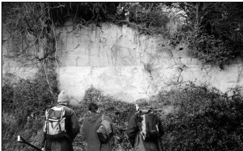
Figure 4. Exposure of brickearth at Pegwell Bay, with the darker decalcified horizon overlying the paler unleached material that has the calcite needles bridging between the silt particles.
