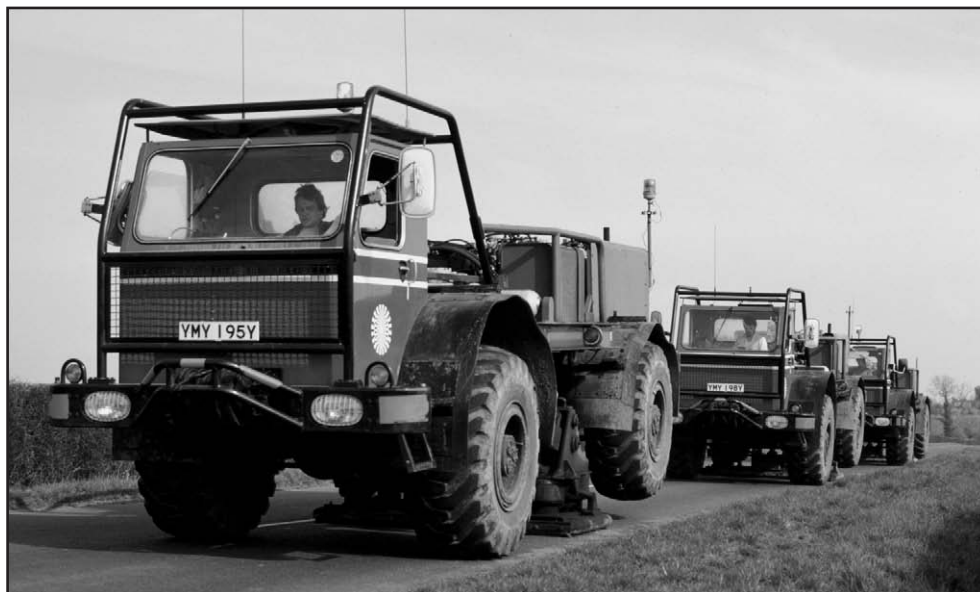
Geophysical exploration with Vibroseis on a country road near Radcliffe on Trent.
