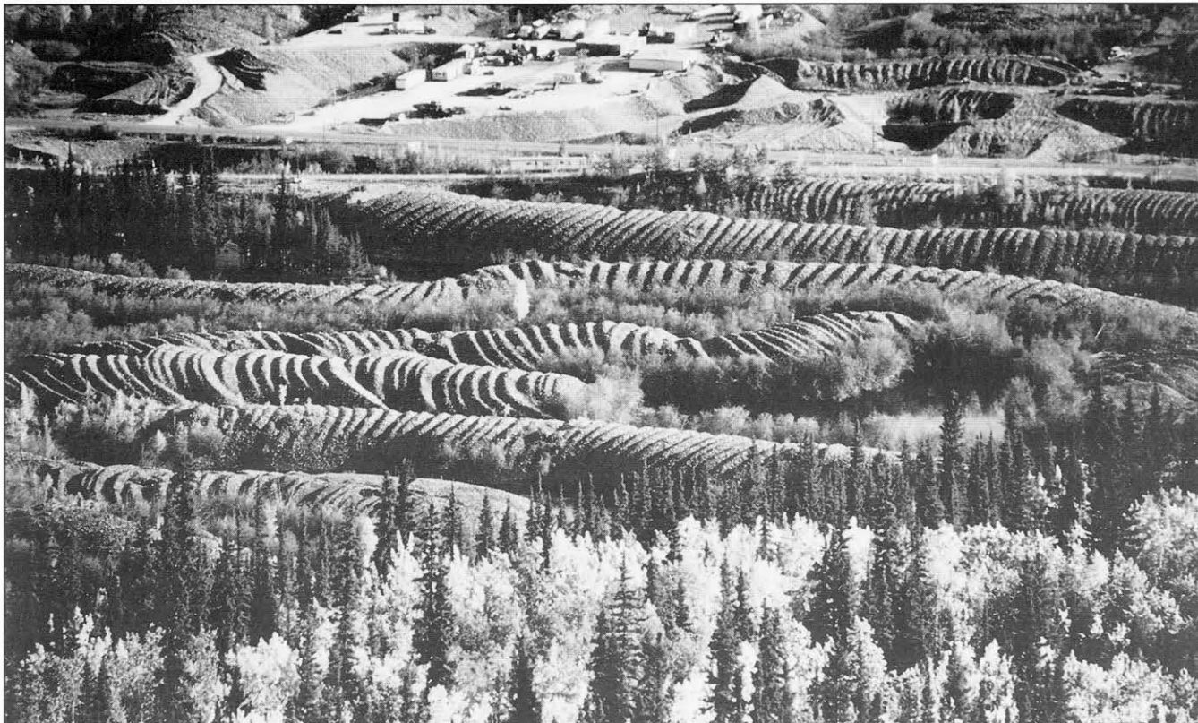
Fig. 11. Characteristic ribbed ridges of dredge tailings on the floor of the Klondike Valley, just upstream of the Bonanza Creek confluence. Some tailings ridges in the background have been regraded to allow re-use of the land as industrial units (photo by the author).
